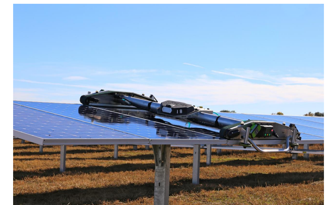
Robotic washer cleans panel at UC Davis Solar Farm, courtesy Sun Power
